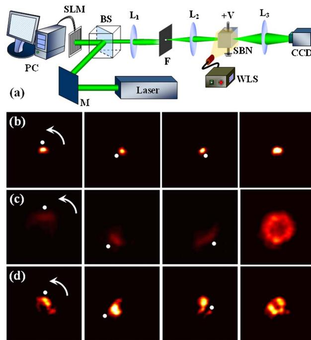
Fig. 3. (Color online) (a) Experimental setup. SLM, spatial light modulator; BS, beam splitter; F, spatial filter; WLS, white-light source. (b) Single-blade propeller generated in experiment corresponding to Fig. 1(b). Four panels are snapshots of three instantaneous patterns plus the time-averaged intensity pattern at input; (c) and (d) depict output patterns after (c) linear diffraction and (d) nonlinear self-trapping through the crystal, corresponding to Fig. 2 (Media 3, 48.1 KB).
