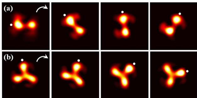
Fig. 4. (Color online) Experimental generation of optical propellers with (a) two and (b) three blades corresponding to the numerical results shown in Figs. 1(c) and 1(d). Four snapshots are taken from a movie shown online (Media 4, 212 KB).
